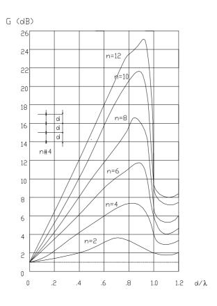
Gains diagram of horizontal dipole Array with "n" dipoles versus relative  $D/\lambda$  distance between them
