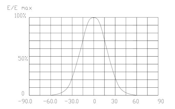
On a second diagram, set the distance in function of the vertical angle of the points indicated before (Fig.4). By linking these new points, you obtain the shape that the vertical pattern should have. In practice, in order to avoid that the areas situated under higher vertical angles, it is possible to have reflections caused by the power which is radiated on the maximum.
