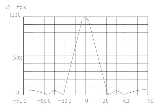
The optimum spacing between the elements in this type of distribution is 0,5 2  $\lambda$  even if in real practise bigger spacings are used.
