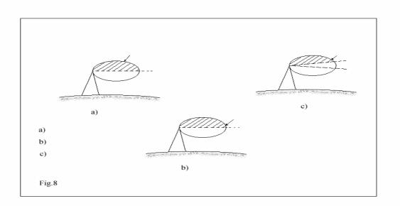
The pattern of an antenna situated at 300 meters from the earth will have to be beam tilted of an angle superior to 0.5 degrees in order to enable the maximum radiation to reach the earth surface.
