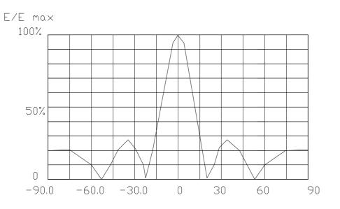
Vertical radiation pattern of a curtain composed of elements with a space of  $0.5\lambda$ . between each other and feeder with the same current and phase.
